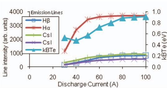
FIG. 6. (Color online) Optical emission peaks vs pulsed discharge current.
