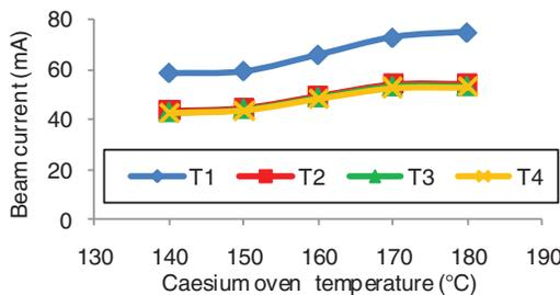
FIG. 7. (Color online)  $H^-$  beam currents vs caesium oven temperature for a 55 A discharge.
