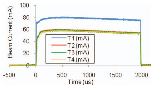
FIG. 9. (Color online) Beam current profiles of 60 mA at 25 Hz. (2.2 ms, 64 A discharge, 19.6 kV extraction voltage, 65 keV beam, 190 °C caesium oven, 16 mLmin<sup>-1</sup> H<sub>2</sub>.)
