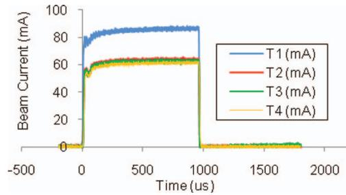
FIG. 8. (Color online) Beam current profiles of 62 mA at 50 Hz 1 ms. (1.2 ms, 60 A discharge, 19.6 kV extraction voltage, 65 keV beam, 180 °C caesium oven, 16 mLmin<sup>-1</sup> H<sub>2</sub>.)
