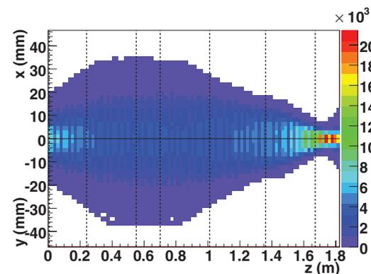
FIG. 5. (Color online) The  $x$  and  $y$  envelope of the beam along the length of the LEBT, up until the location of the RFQ entrance, based on the GPT simulation results for the nominal solenoid settings (137 A, 123 A, 216 A). Here  $z = 0$  is near to the location of the first toroid (T1 in Fig. 1), while the dotted vertical lines show the boundaries of the solenoids.
