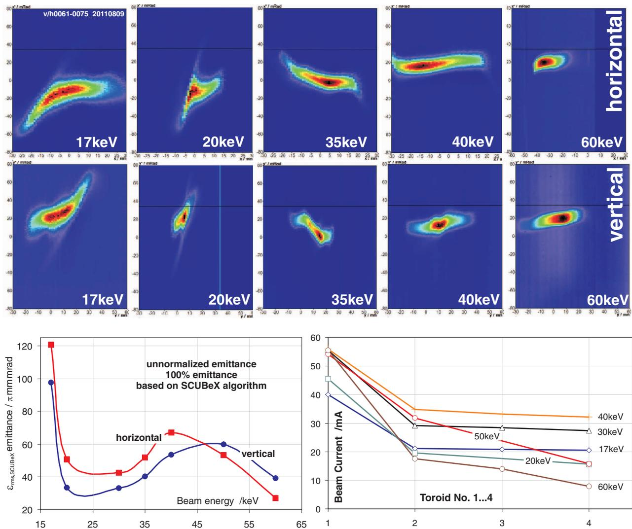
FIG. 3. (Color online) Variation of the beam energy vs. rms emittance and beam current, all three solenoids are constant at 70 A. The scanning range is for both  $x'$  and  $y' \pm 80$  mrad and for  $x = \pm 30$  mm and for  $y = -30 \dots +60$  mm. The lowest possible beam energy is the extraction voltage of 17 kV.
