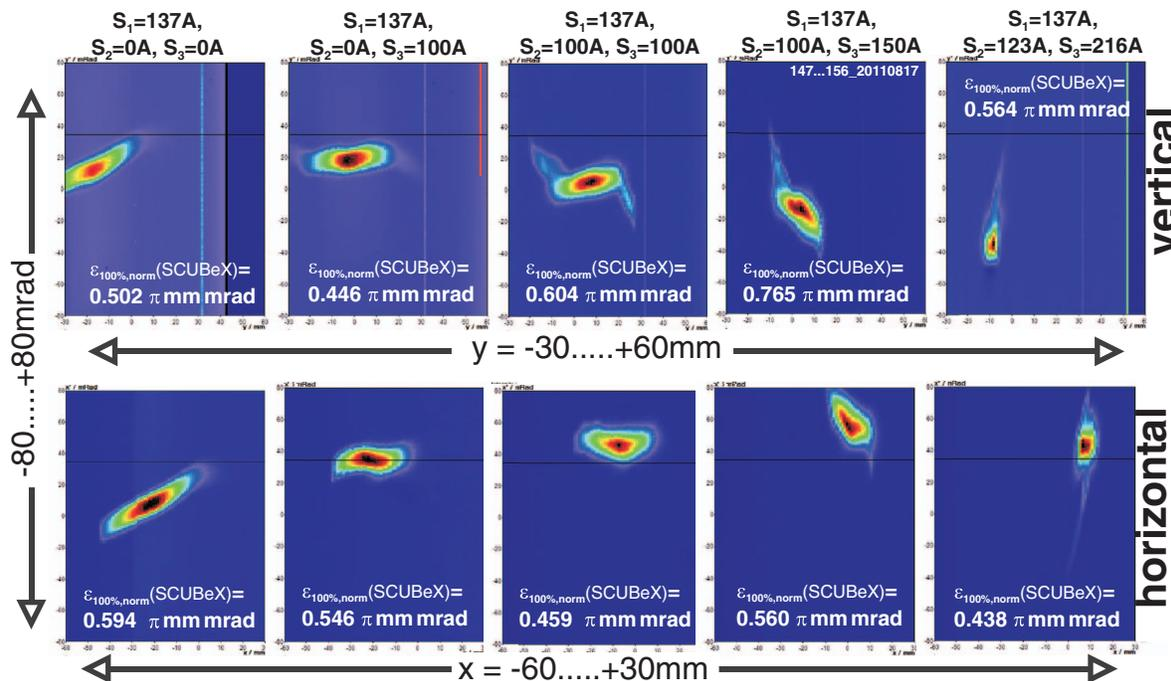
FIG. 2. (Color online) Horizontal and vertical emittances for a 65 keV beam with fixed B-field for S1 and increasing magnetic field from left to right, note the beam offset in both planes. The chosen setting for S1 is so that the measured beam current values along the LEBT only show marginal losses. The two scanner cover a different range in  $x$  and  $y$ .
